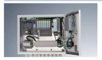
IntelliRamp® is the recently developed control system performing braking processes reproducably with the variables speed versus time
