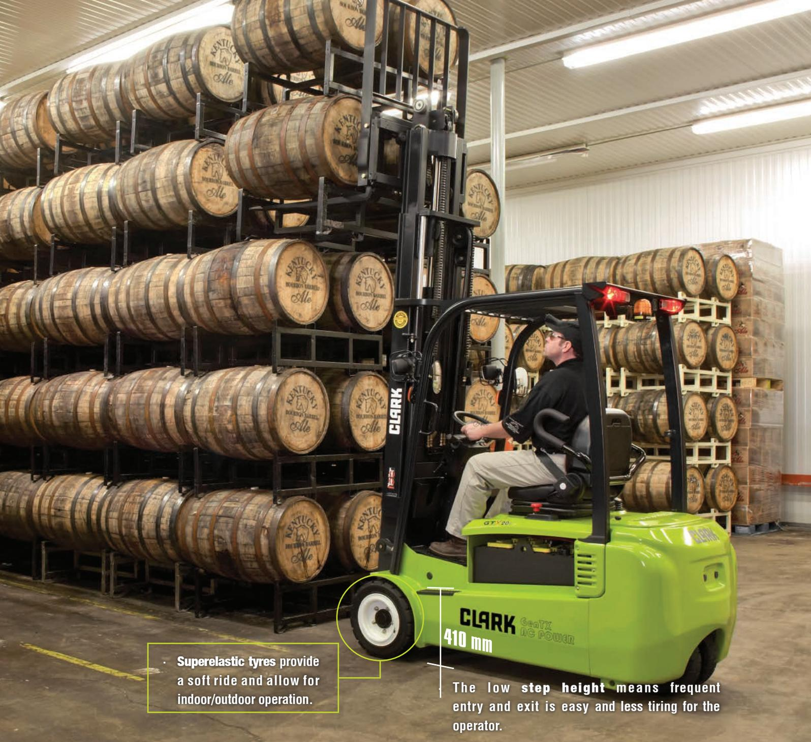
Superelastic tyres provide a soft ride and allow for indoor/outdoor operation.
